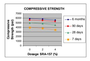
In mix designs incorporating **SRA-157**, compressive strengths may be slightly less than normal. It is reasonable to expect a 5% - 10% strength loss, but this is usually not an issue. For mixes where strength must be maintained, a mid-range water reducer such as
