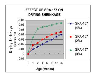
Mix designs incorporating **SRA-157** will significantly reduce drying shrinkage, consequently reducing or possibly eliminating drying shrinkage cracks.
